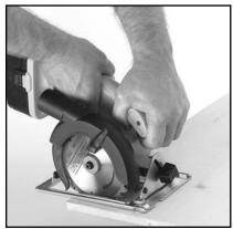
Fig 9. Proper Holding Grip.
